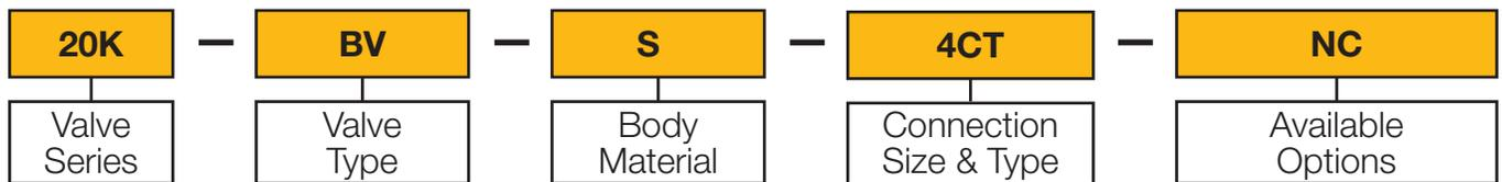
Describes a 20K Ball Valve in stainless steel construction, equipped with 1/4" Cone & Thread inlet and outlet. Supplied with NACE Certification.
