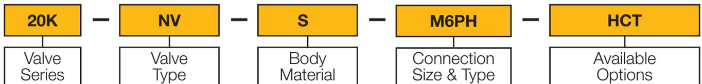
Describes a 20K Needle valve in stainless steel construction, equipped with 6mm Phastite® inlet and outlet. Supplied with Heat Code Traceability marking on all wetted parts.
