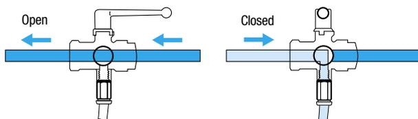
With vent connected to a silencer = noiseless discharge to atmosphere
