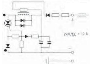
These electrical parts need an external fuse of I = 100 mA
