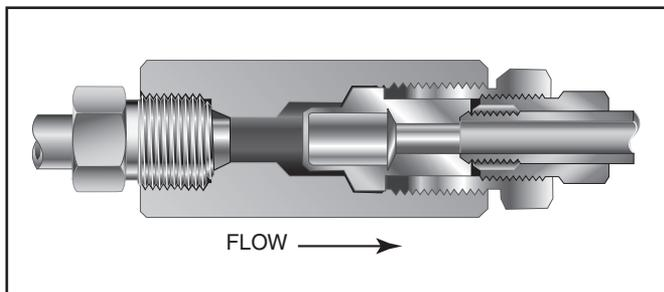
Parker Autoclave Engineers High Flow Cup-Type Line Filters are recommended in high pressure systems requiring both high flow rates and maximum filter surface area. Widely used in the industrial and chemical processing fields, the cup design offers as much as six times the effective filter area as compared to disc-type units. In addition, the filter elements can be quickly and easily replaced.
