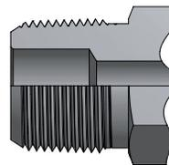
F - ANSI/ASME B1.20.1 Internal pipe threads
