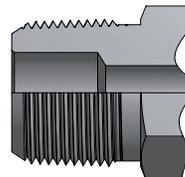
F - ANSI/ASME B1.20.1 Internal pipe threads
