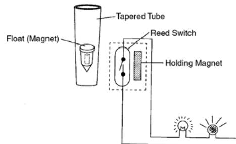
Caution must be taken when mounting multiple alarmed meters. Close proximity may cause interference with alarm signal.
