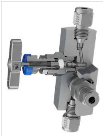
HNV series gauge vent hand valve with inverted tube fitting to inlet and outlet connections with Parker PTFree connect™ tube fitting connection to the vent.
